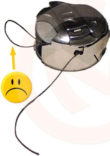
The braking of the bobbin is therefore much in use with sewing machines equipped with thread trimming devices, high stitching speeds, and in all cases where bobbins present high inertial forces.
