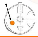
In this execution the braking of the bobbin is achieved by a magnet (1) imbedded into the inside bottom of the bobbin case. This magnet attracts the bobbin and creates friction between the bobbin and the inside bottom of the bobbin case. In order for such braking system to work properly, it is essential to use bobbins made of steel material!
