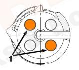
The braking effect of the bobbin is achieved by a magnet (1) embedded into the inside bottom of the basket. This magnet attracts the bobbin and creates friction between the bobbin and the inside bottom of the basket. In order for such braking system to work properly, it is essential to use of bobbins made of steel material!
