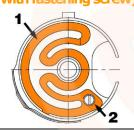
The device consists of a spring (1) embedded on the inside bottom of the bobbin case and fixed by a screw (2) against accidental lost. The spring pushes on the upper flange of the bobbin and the latter against the bottom of the basket, causing a braking effect. The shape of the embedded spring changes according to the different bobbin cases on which it is mounted.
