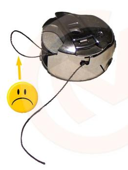
The braking of the bobbin is therefore much in use with sewing machines equipped with thread trimming devices, high stitching speeds, and in all cases where bobbins present high inertial forces.
